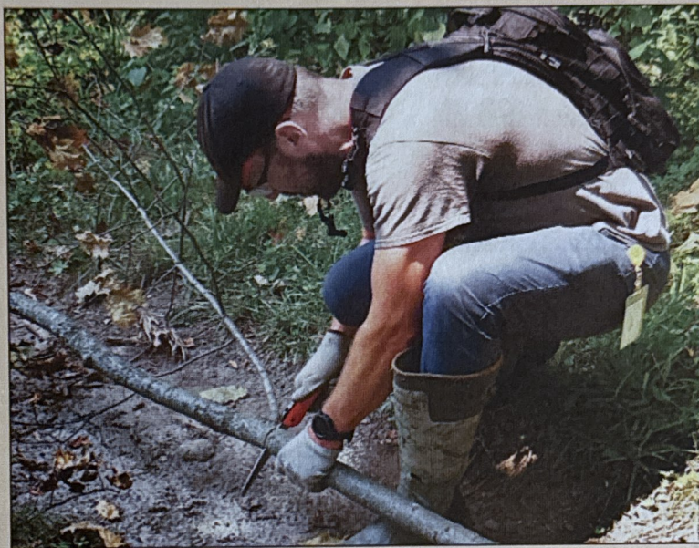
A hand saw is used to cut sections of wood from a wilting tree branch for oak wilt testing.
