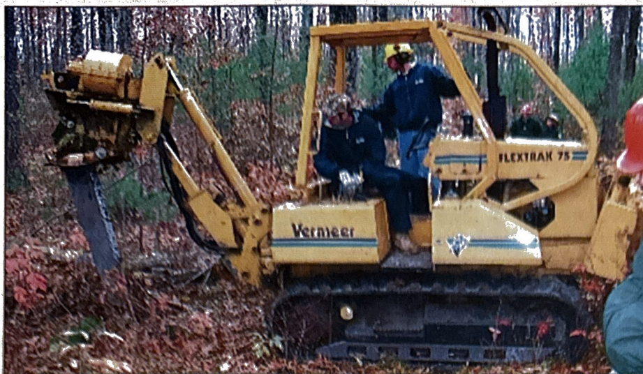
A vibratory plow with a large blade is used to cut roots below ground to stop the spread of oak wilt.
